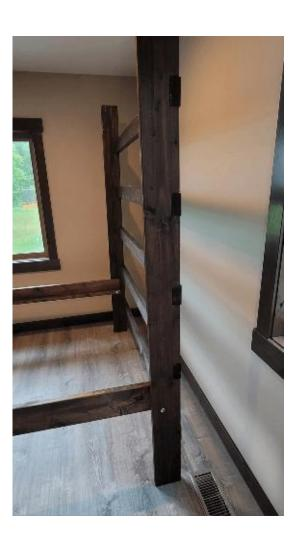
From the back insert one 5.25 In. carriage bolt into the hole of each back leg. Lay the ladder ends on their backs as shown on right. Lay the back rail between the ladder ends. The back rail is positioned with the shorter side above the bolts and the longer side below the bolts. Place a washer, lock washer and nut on each of the bolts and loosely hand tighten the nuts..
